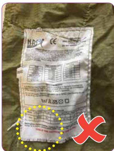
The label has started to fray and therefore the sling **cannot** be used.
