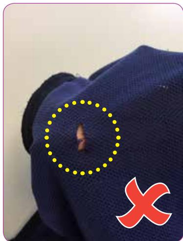
This sling has a hole in the material and the sling **cannot** be used.
