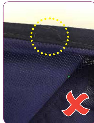
The stitching on the main part of the sling is undone therefore the sling **cannot** be used.
