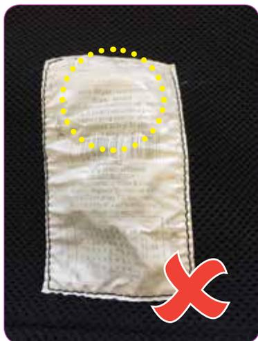
This sling cannot be used as the weight limit and serial number **cannot** be read.
