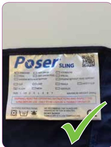
The label can be read easily with the size and weight limit clearly visible. This sling **can** be used.
